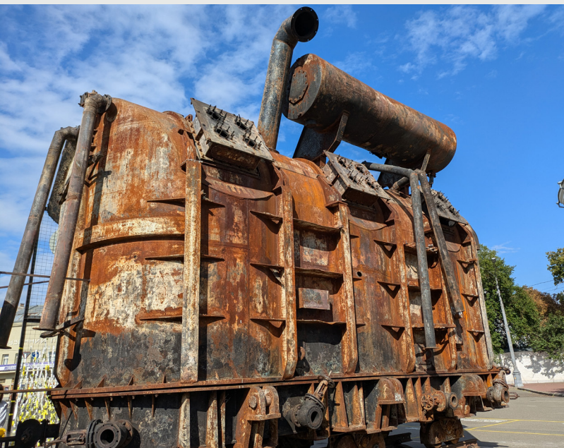
A destroyed power transformer from Burshtynska thermal power plant displayed on a square in Kyiv. Ukraine no longer produces such transformers making them difficult to replace. Photo captured by Physicians for Human Rights in September 2024.
